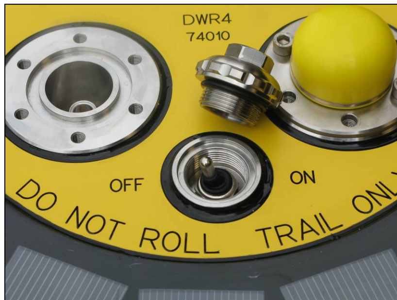
Figure 21.1. External power switch on the hatchcover, underneath the nut with sealing ring and ON and OFF labels on the sides.
