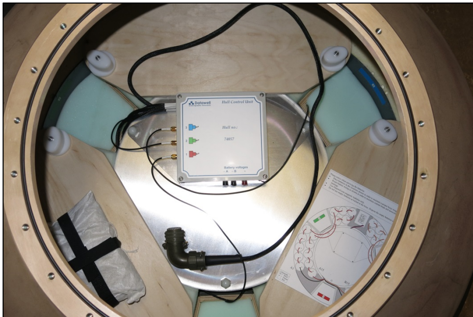
Figure 8.2. ACM electronics inside the hull control unit and coaxial cables of the three acoustic transducers.
